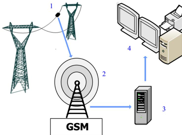
**Figure 3: AL temperature monitoring structure:**
