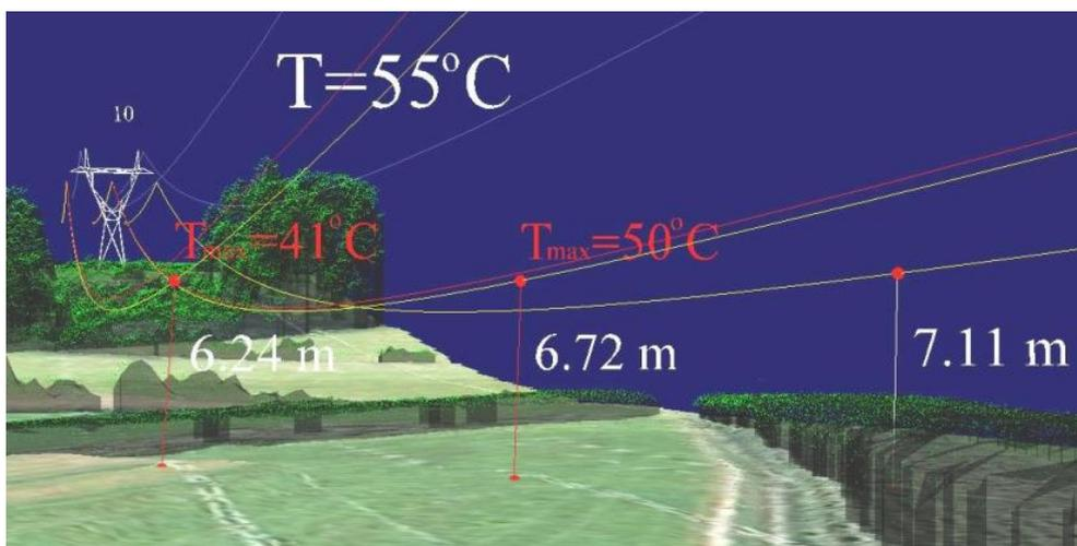
**Figure 2: 3D model of power line**
